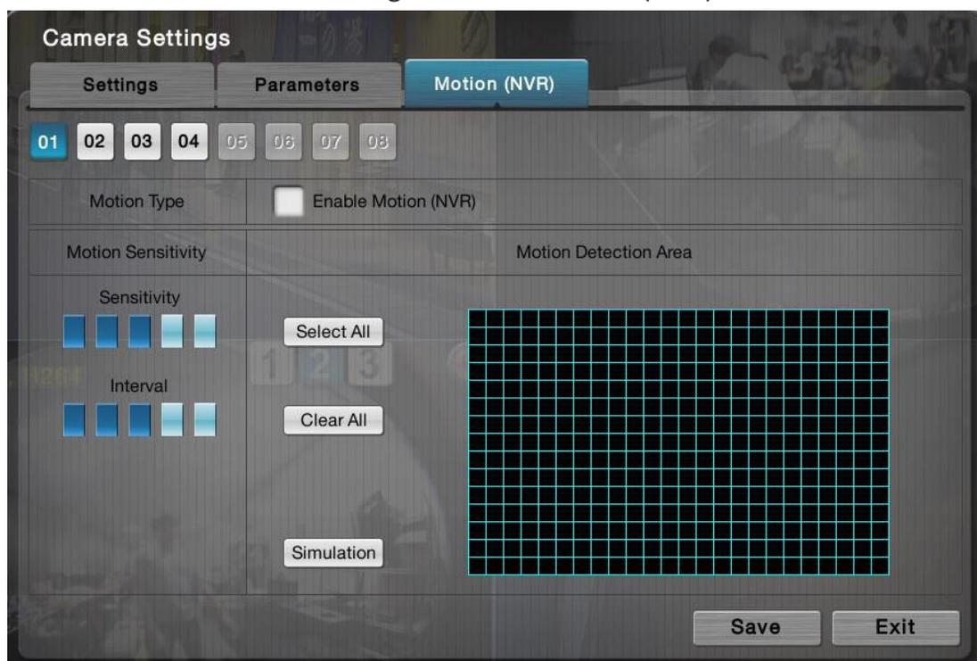
**Step2:** Check the “Enable Motion(NVR)” box, and video from the camera will appear. Then set up motion detection’s sensitivity, interval, and detection area.
