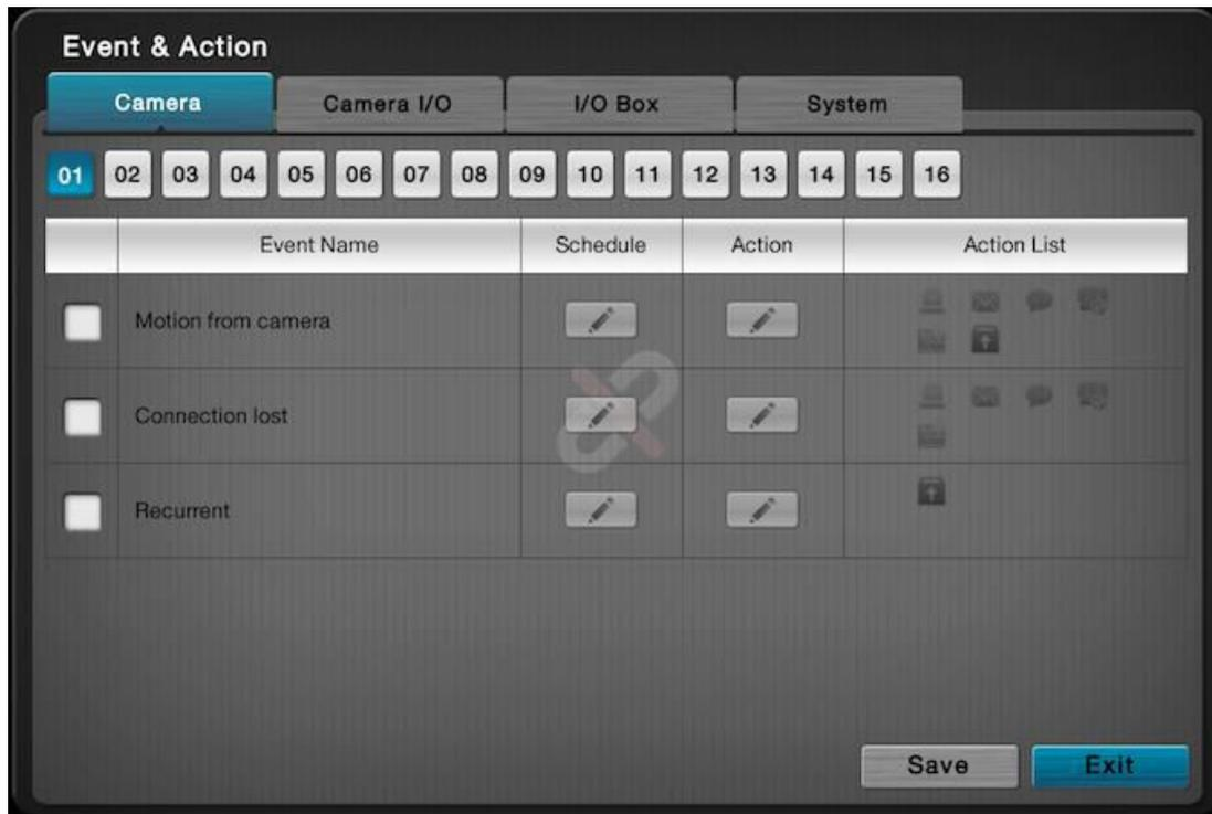
**Step2:** Check the “Motion from camera” box and edit the schedule and actions, which including “Output”, “Email”, “Push Notification” and so on. Then you will see the corresponding actions when motion alarm is triggered.
